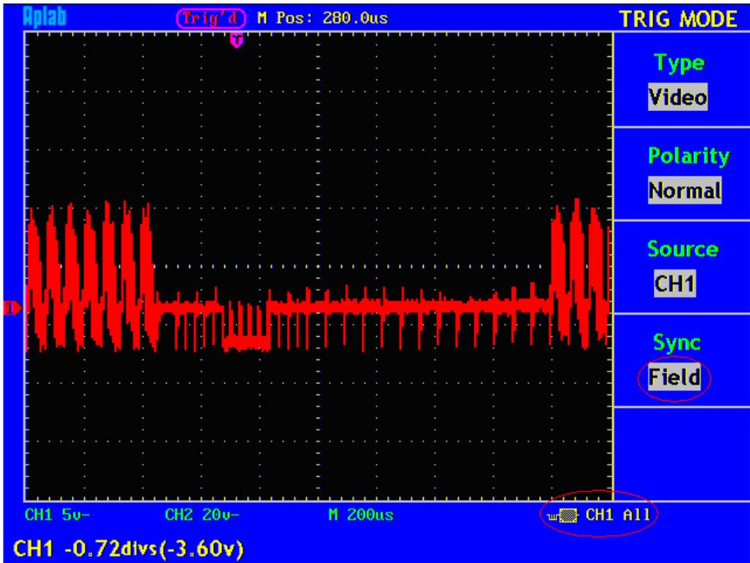
Fig. 31 Wave Form Triggered in the Video Field
