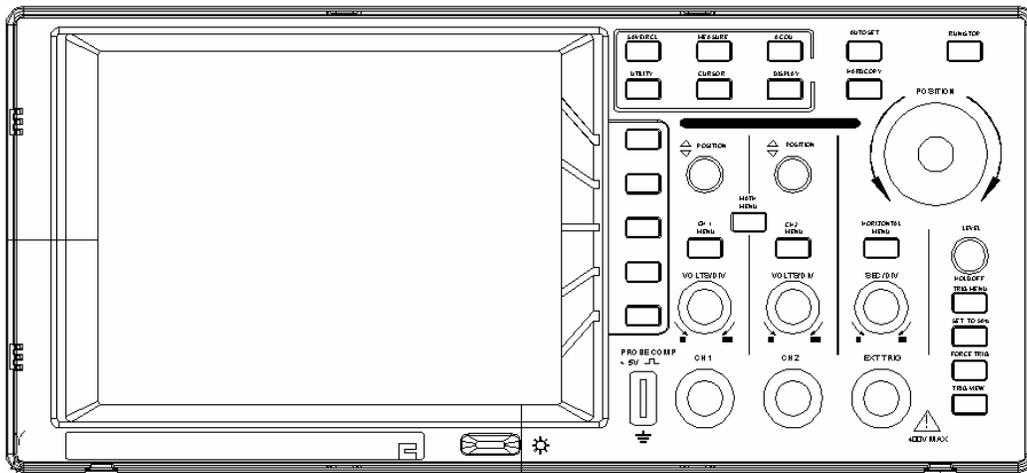
**Fig. 1** The Front Panel of a Digital Storage Oscilloscope
