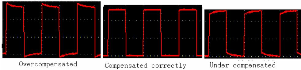
**Fig. 7** Displayed Wave Forms of the Probe Compensation
