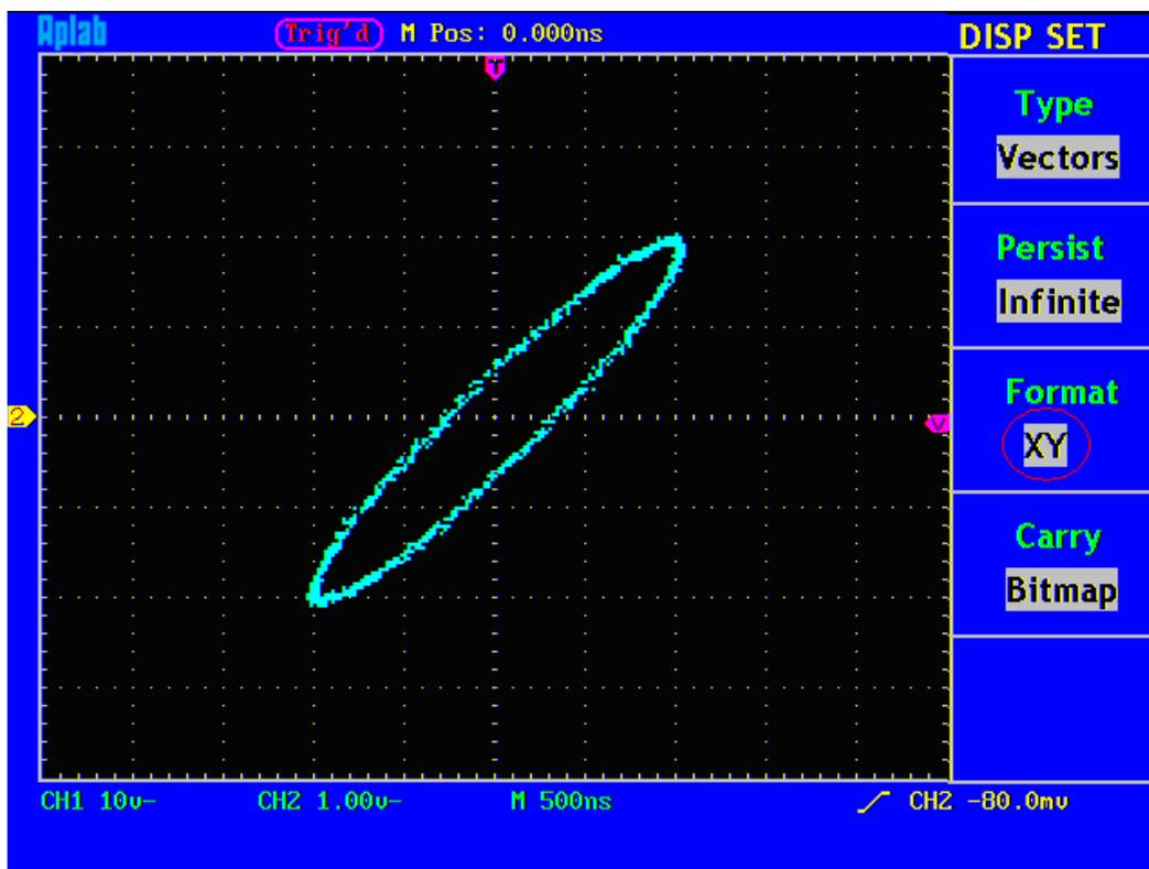
**Fig. 41** XY Display Mode
