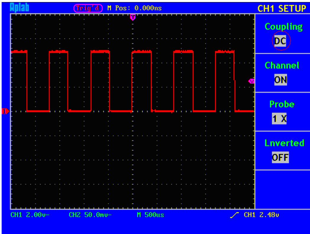
Fig. 16 “DC Coupled” Oscillogram
