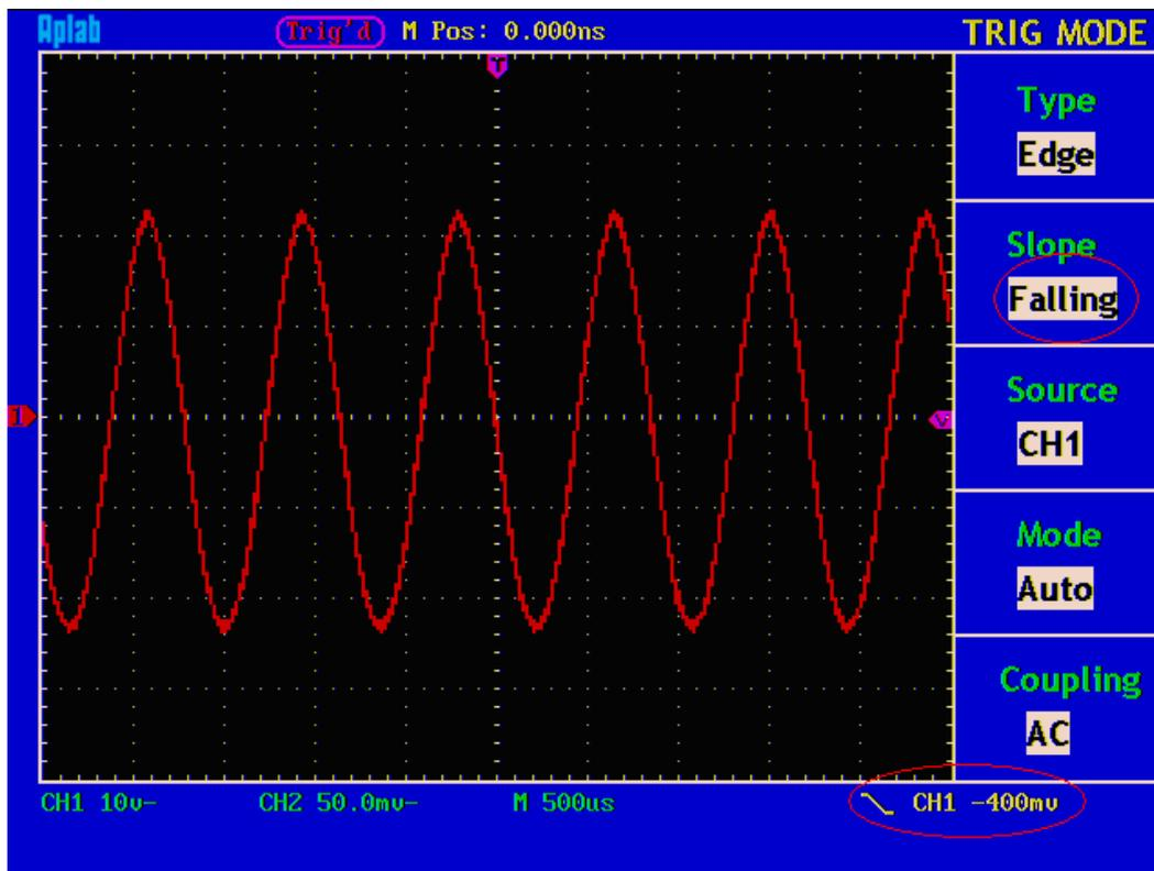
Fig. 29 Wave Form Triggered on the Falling Edge
