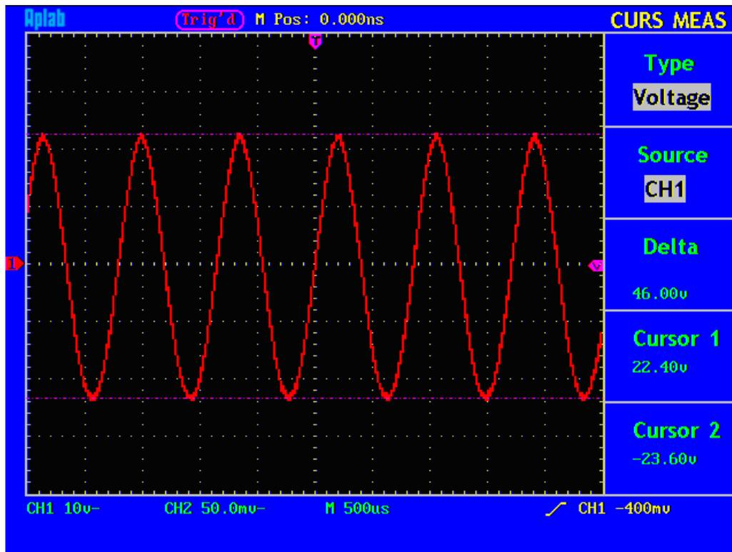
**Fig. 51** Wave Form of Voltage Cursor Measurement
