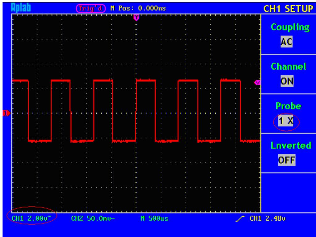
**Fig. 17** Adjusting the Attenuation Ratio of the Probe
