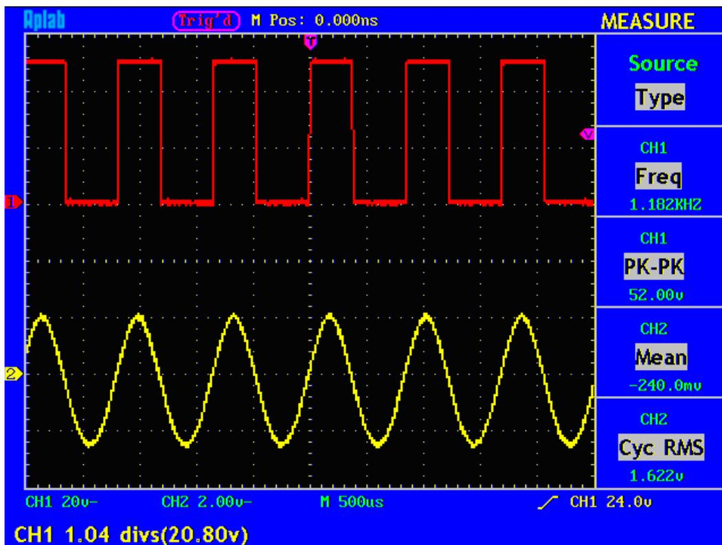
Fig. 49 Automatic Measurement
