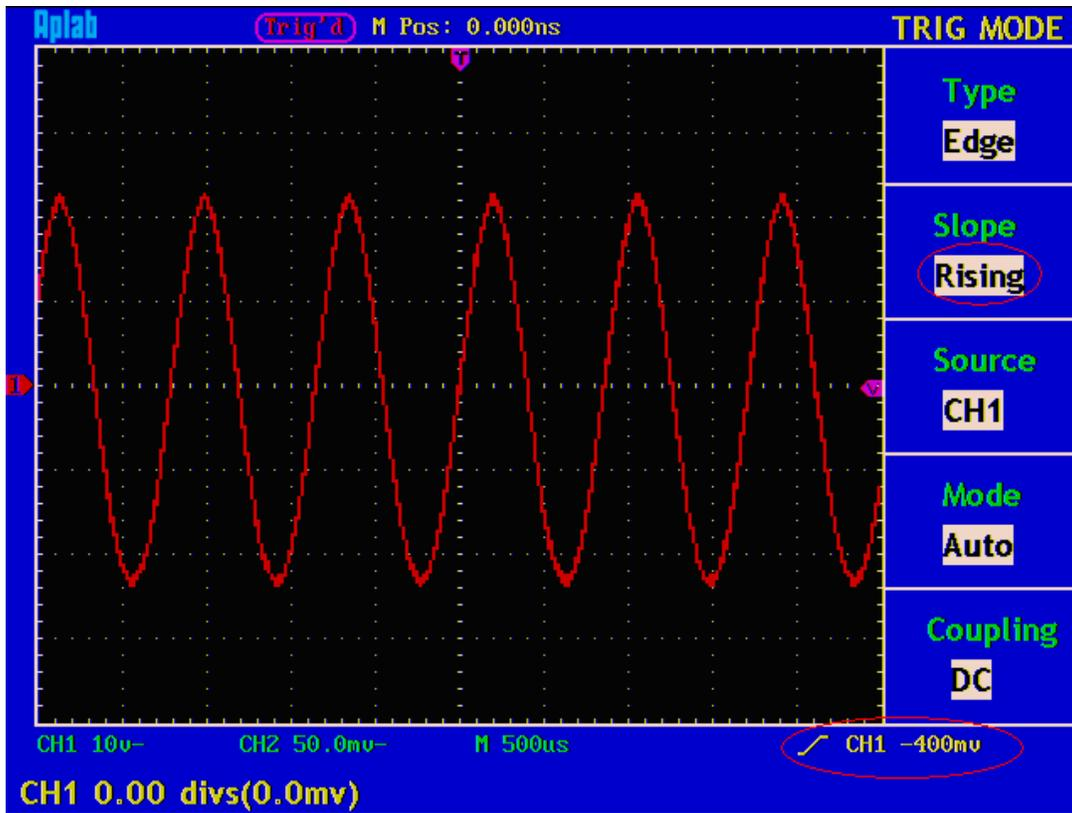
Fig. 28 Wave Form Triggered on the Rising Edge
