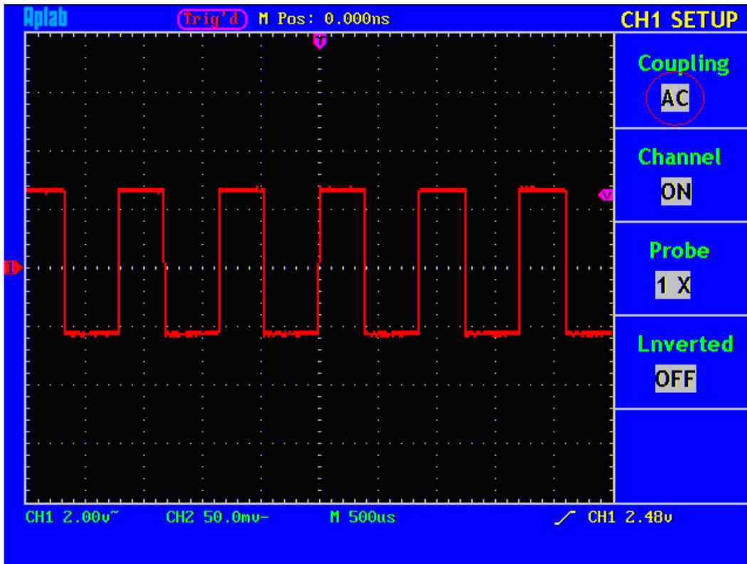
Fig. 15 An “AC Coupled” Oscillogram
