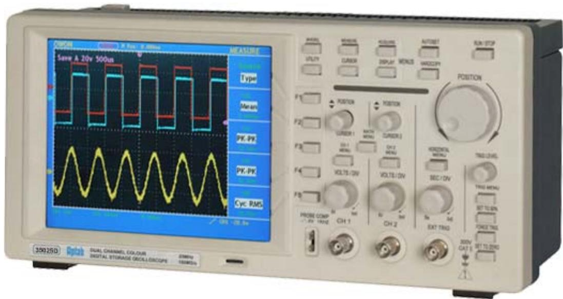
**Portable Colour Digital Storage Oscilloscope**
