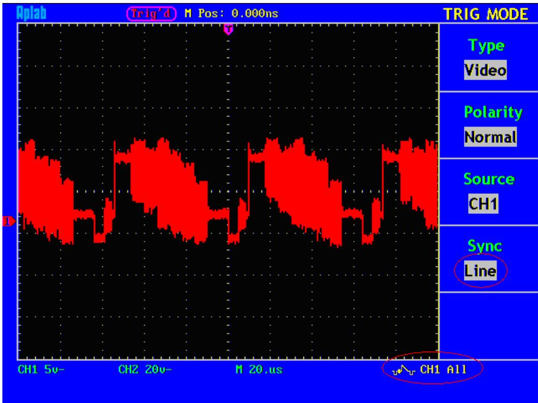
Fig. 32 Wave Form Triggered in the Video Line
